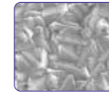
金刚石涂层刀具表层形貌图 Surface picture of diamond coating tool
